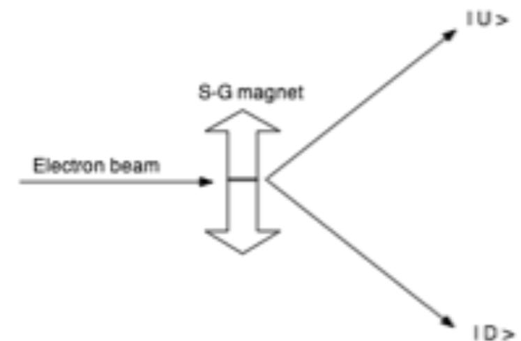
Ask if experimental results  $\rightarrow$  genuinely measuring some state property(U/D) of electrons, or if magnet is simply randomly deflecting them one way or other. Answer question by modification of experiment - electron detector removed/replaced by further pair of S-G magnets arranged so that electrons passing out of first magnet pass through one of two further magnets
