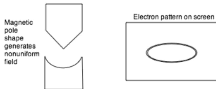
Hypothetical experiment to see how much deflection takes place when pass electron beam between poles magnet. Detect deflected electrons outside field region; Can detect single electrons.
