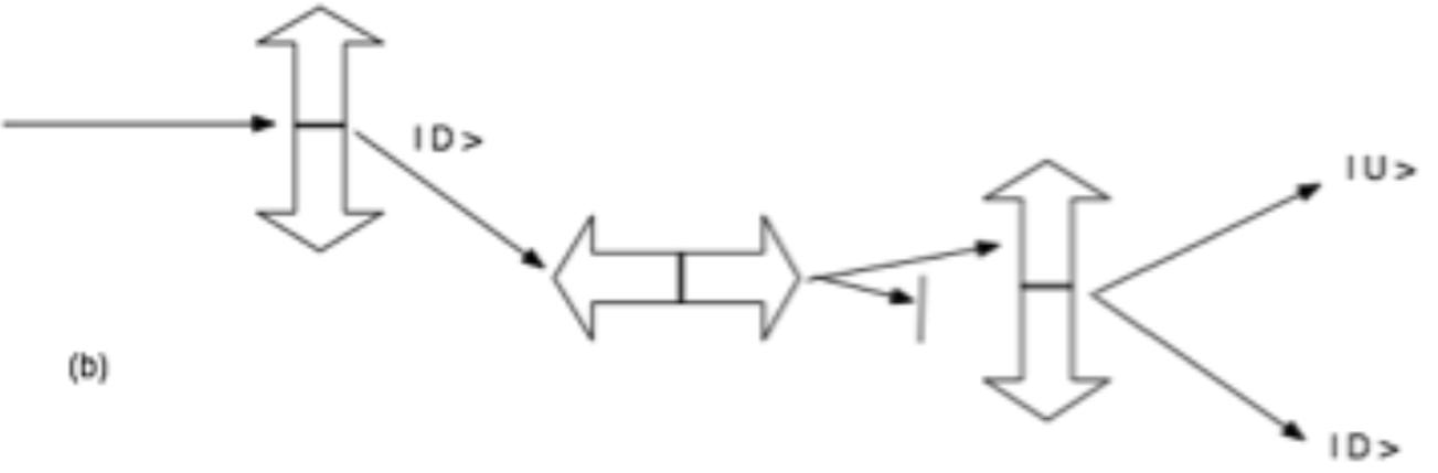
(b) Blocking LEFT channel produces mixture of  $|U\rangle/|D\rangle$  states in electrons that pass through RIGHT channel.
