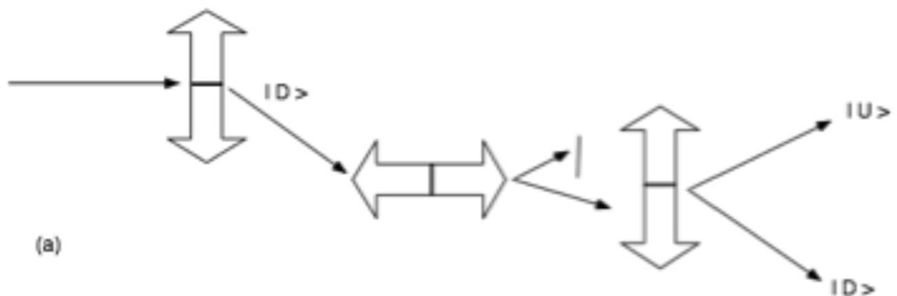
(a) Blocking RIGHT channel produces mixture of  $|U\rangle/|D\rangle$  states in electrons that pass through LEFT channel.
