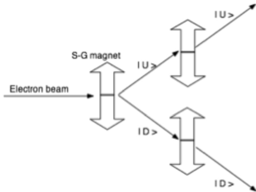
Results(corresponds to repeatability measurements) are conclusive. Electrons that emerge along UP channel of first magnet then pass through topmost second magnet and all emerge from that magnet's UP channel.
