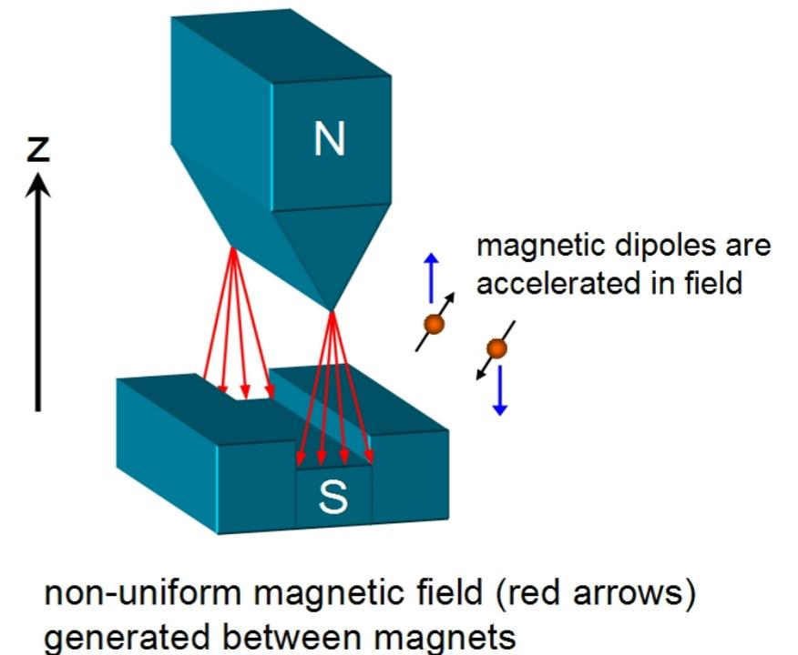
non-uniform magnetic field (red arrows) generated between magnets
