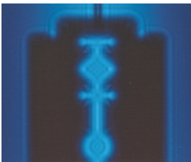
FIGURE 37-2 ■ The diffraction pattern produced by a razor blade in monochromatic light. Note the lines of alternating maximum and minimum intensity.
