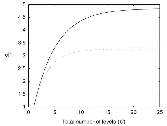
**Fig. 2.** Dependence of the quantity  $S_3 = \sum_{k=1}^C [1/(N_k)^{\frac{1}{3}}]$  on the total number of levels,  $C$ , for two networks. Solid curve: a network where at each node the number of vessels doubles ( $v_k = 2$  for all  $k$ ). Dotted curve: a network where at each node the number of vessels triples ( $v_k = 3$  for all  $k$ ). Note the small linear scale at the y-axis which implies that even for small  $C$  the dependence of  $S_3$  on  $C$  and hence on  $M$  is negligible.
