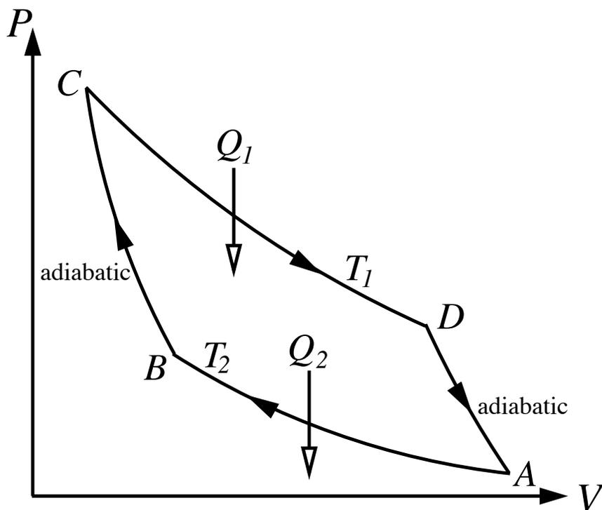
**Figure 3.5:** The Carnot cycle for an ideal gas.
