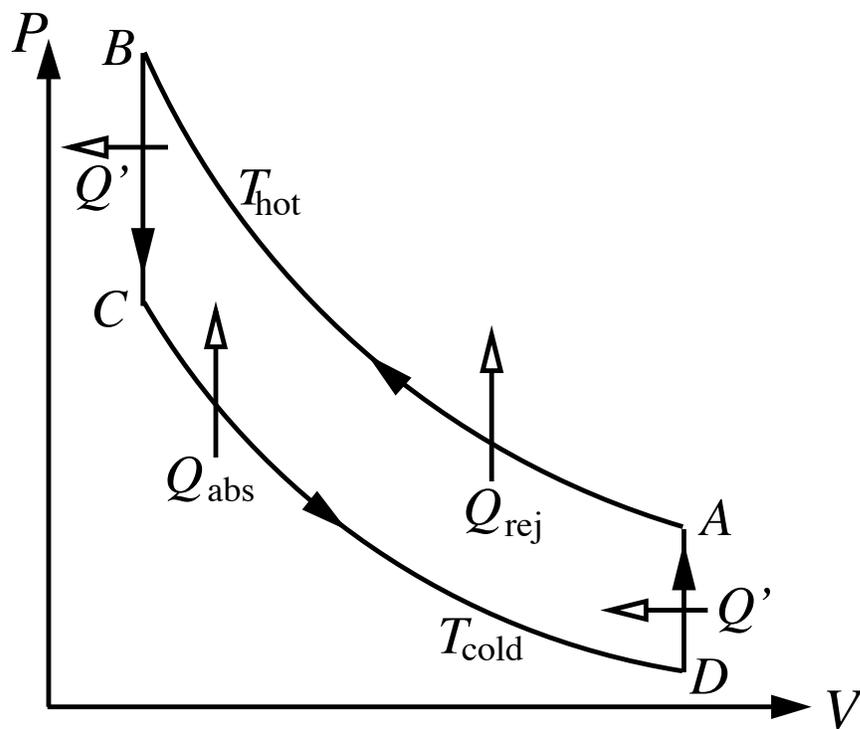
Figure 3.3: The reversed Stirling cycle.
