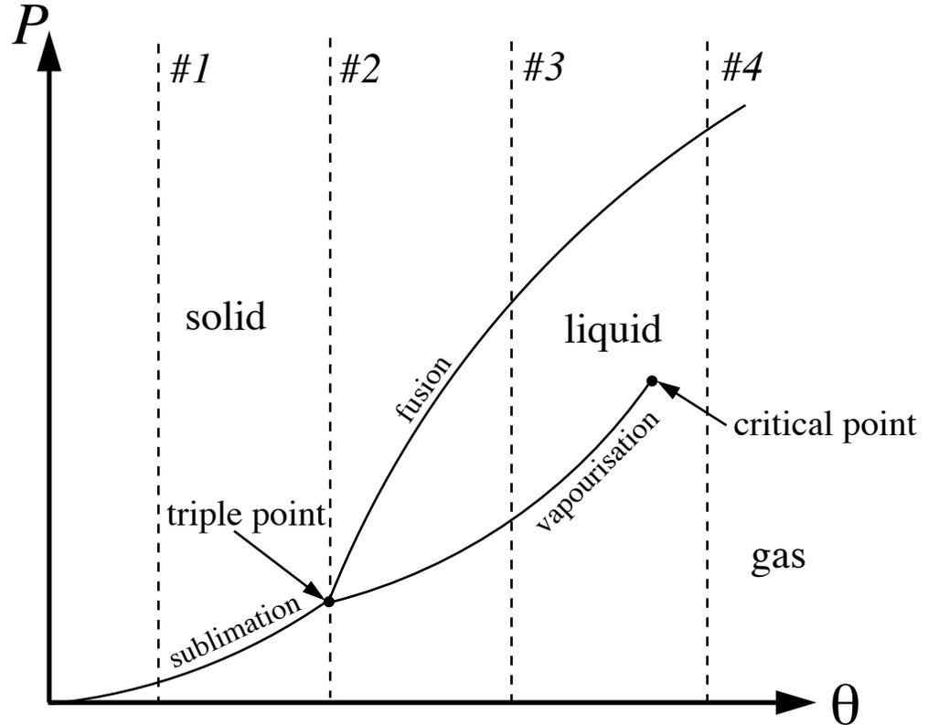
**Figure 1.2: Sublimation curve:** solid and gas states are in equilibrium. **Fusion curve:** solid and liquid states are in equilibrium. **Vapourisation curve:** liquid and gas states are in equilibrium. **Triple point:** solid, liquid, and gas states are in equilibrium. **Critical point:** end point of the vapourisation curve; continuous transition between gas and liquid possible beyond the critical point.
