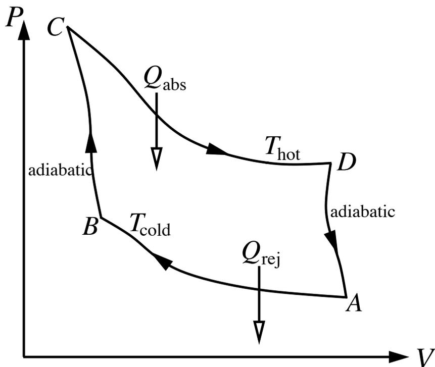
**Figure 3.4:** The Carnot cycle for an arbitrary fluid.
